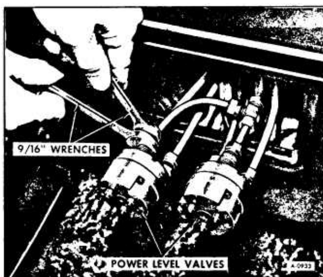
Figure 23—Removing Power Level Valve
