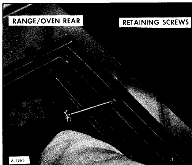
Figure 23—Removing Upper Range/Oven Anchor Screws
