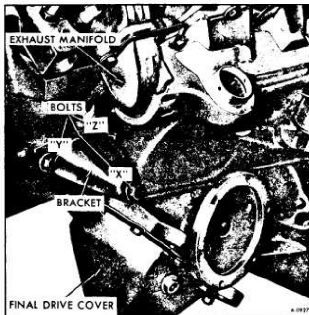
Figure 58—Disconnecting Final Drive From Engine
