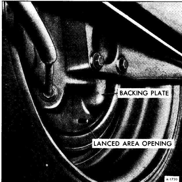
Figure 6—Lanced Area in Backing Plate
