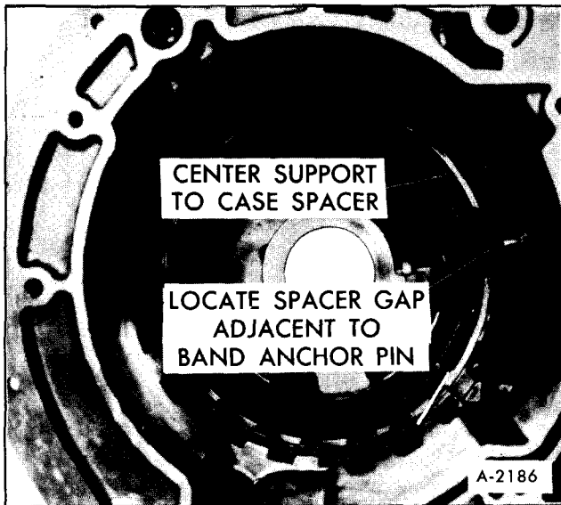
Figure 69—Installing Support-to-Case Spacer
