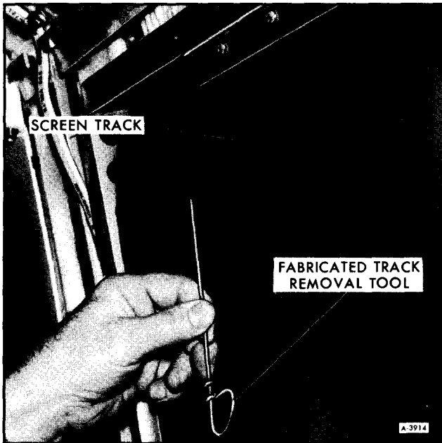
Figure 10—Removing Screen Track
