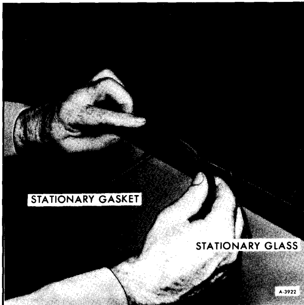
Figure 18—Installing Stationary Gasket
