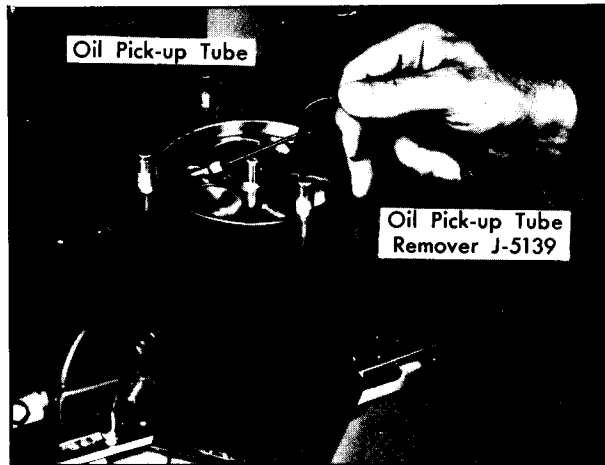
Figure 67—Removing Oil Pick-Up Tube
