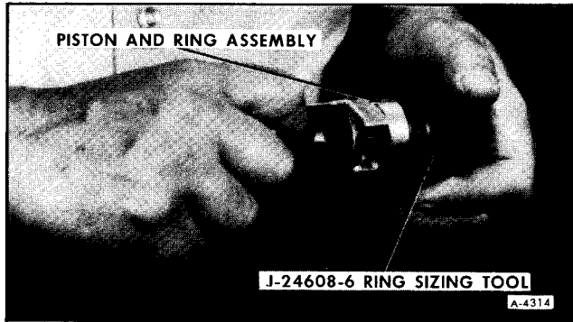
Figure 88—Turning Piston and Ring Assembly into Ring Sizing Tool
