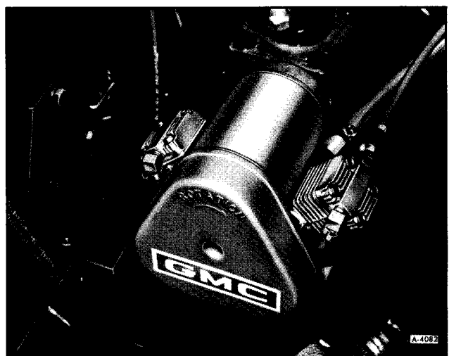
Figure 3—Air Compressor Location (Dana)
