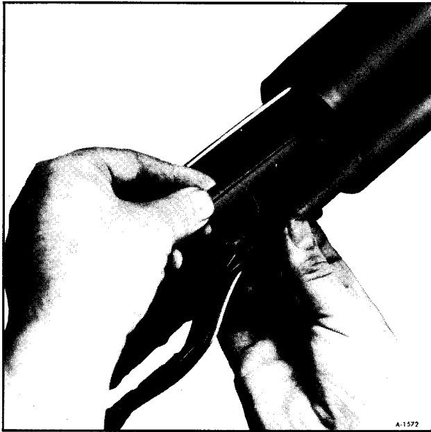
Figure 78—Removing Wire Protector
