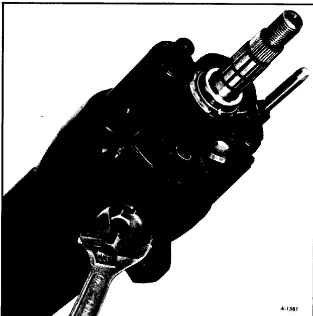
Figure 87—Removing Pivot Pins
