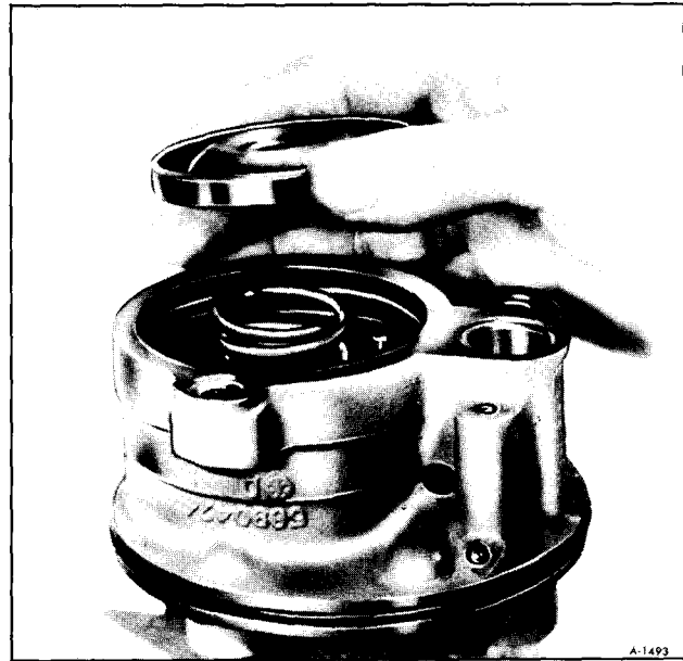
Figure 12—Removal of End Plate
