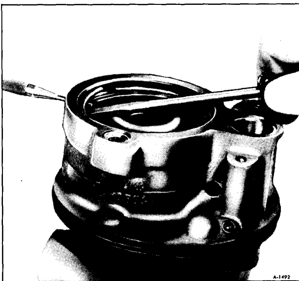
Figure 11—Removal of End Plate Retaining Ring
