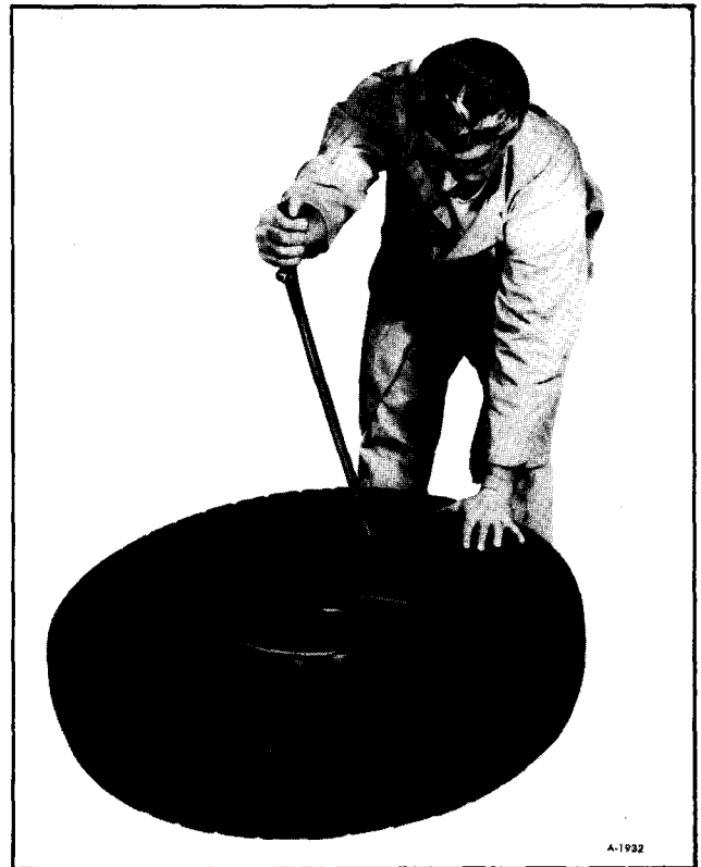
Figure 6—Working Bead Onto Rim
