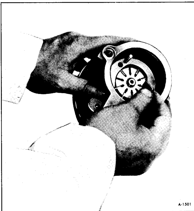
Figure 20—Replacement of Pump Vanes
