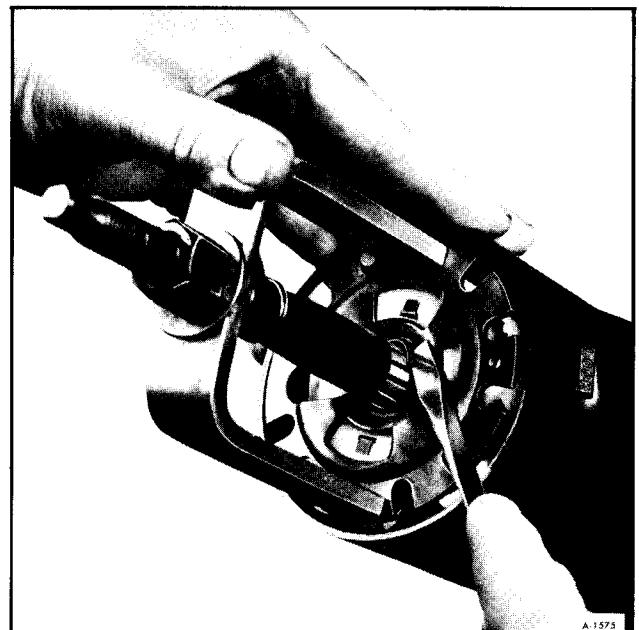
Figure 81—Using Tool to Remove Retaining Ring
