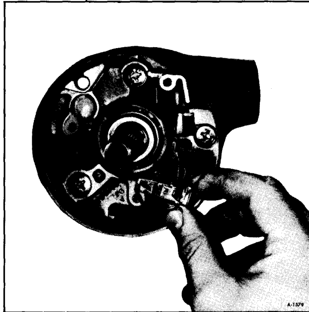
Figure 85—Buzzer Switch and Spring Retainer
