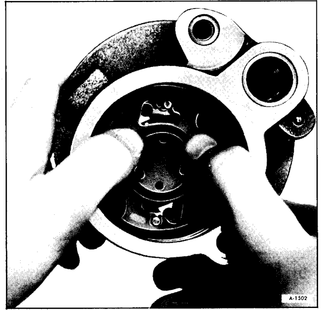
Figure 21—Installing Pressure Plate
