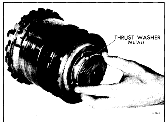
Figure 74—Installing Metal Thrust Washer
