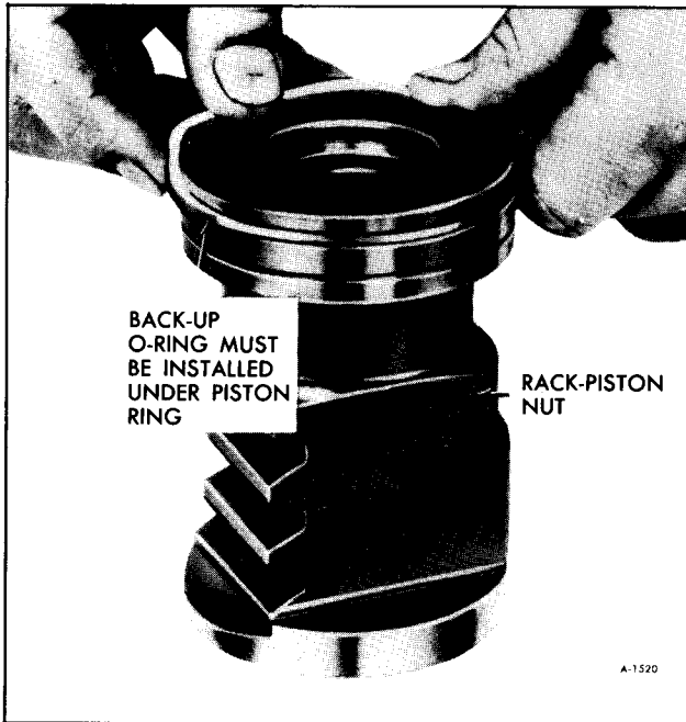
Figure 40—Installing Ring on Rack-Piston
