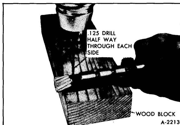
Figure 105—Drilling Governor Gear Shaft
