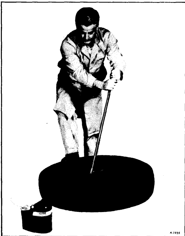
Figure 9—Lifting Bead Over Rim
