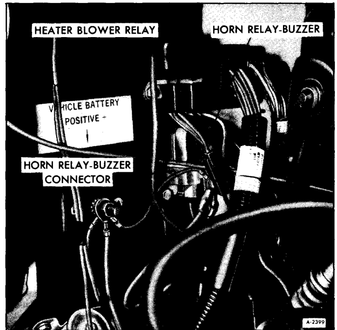
Figure 44—Horn Relay-Buzzer Installation
