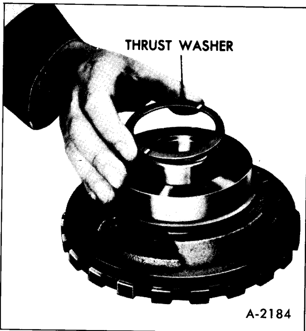
Figure 70—Center Support to Reaction Carrier Thrust Washer
