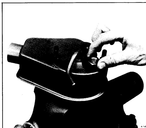
Figure 9—Studs &amp; Union Being Removed
