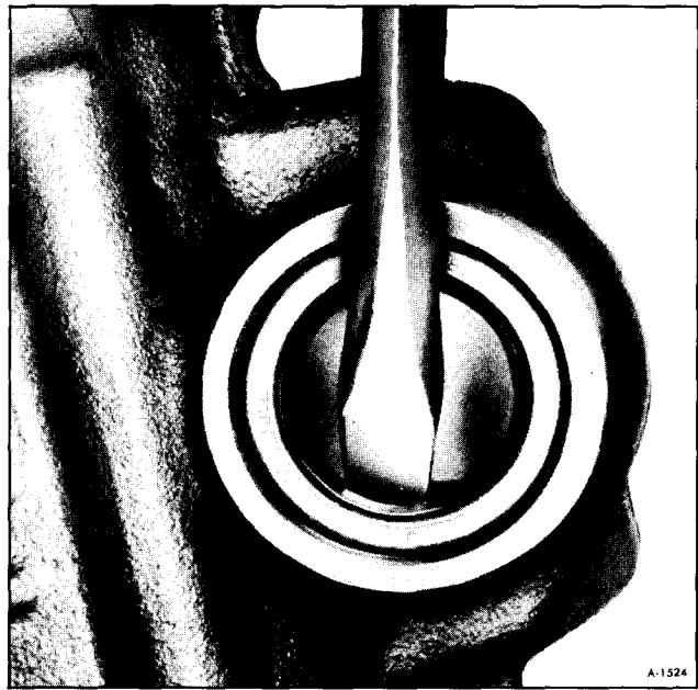
Figure 44—Prying Out Inner Seal
