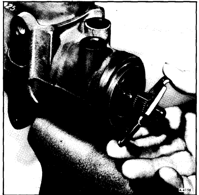
Figure 57—Removing Adjuster Plug Nut
