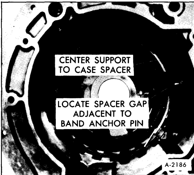
Figure 72—Installing Support-to-Case Spacer
