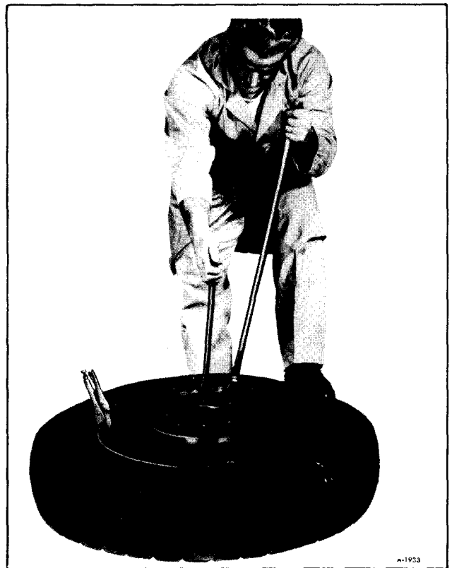
Figure 7—Working Second Bead Onto Rim
