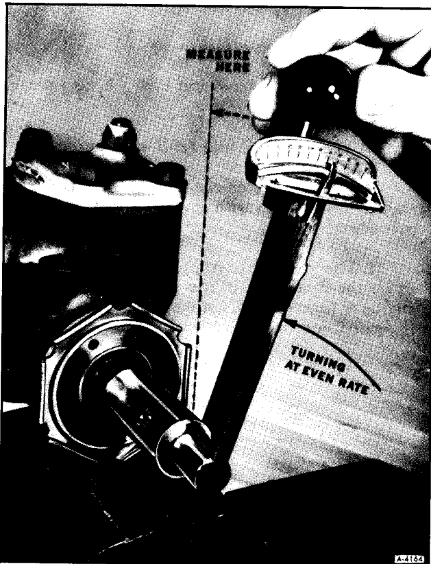
Figure 63—Torque Wrench Reading
