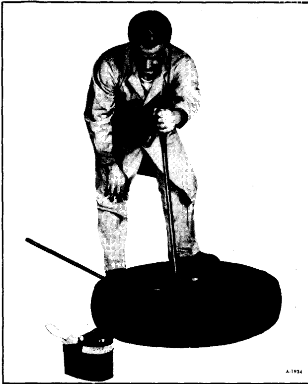
Figure 8—Inserting Tire Iron to Lift Bead
