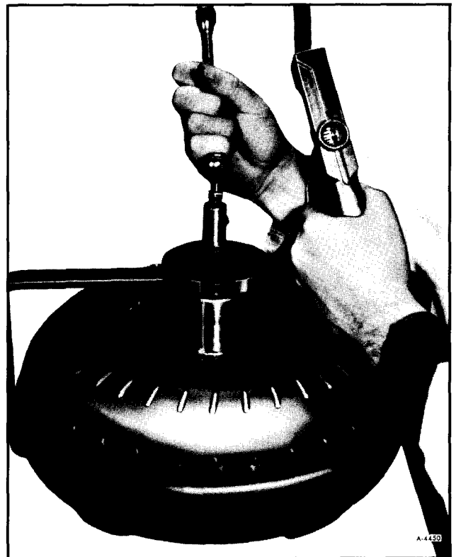
Figure 107—Leak Checking Converter
