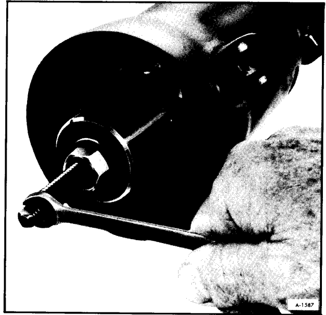
Figure 93—Installing Shift Tube
