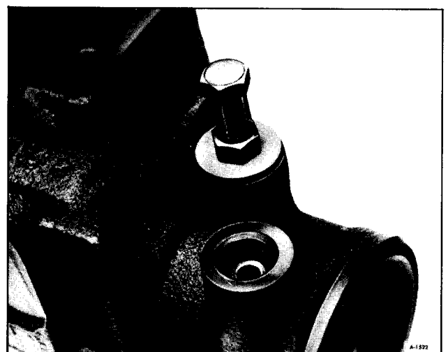
Figure 42—Removing Hose Connector Seat
