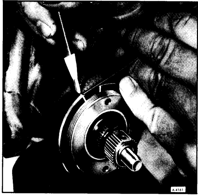
Figure 60—Marking Rotation Distance
