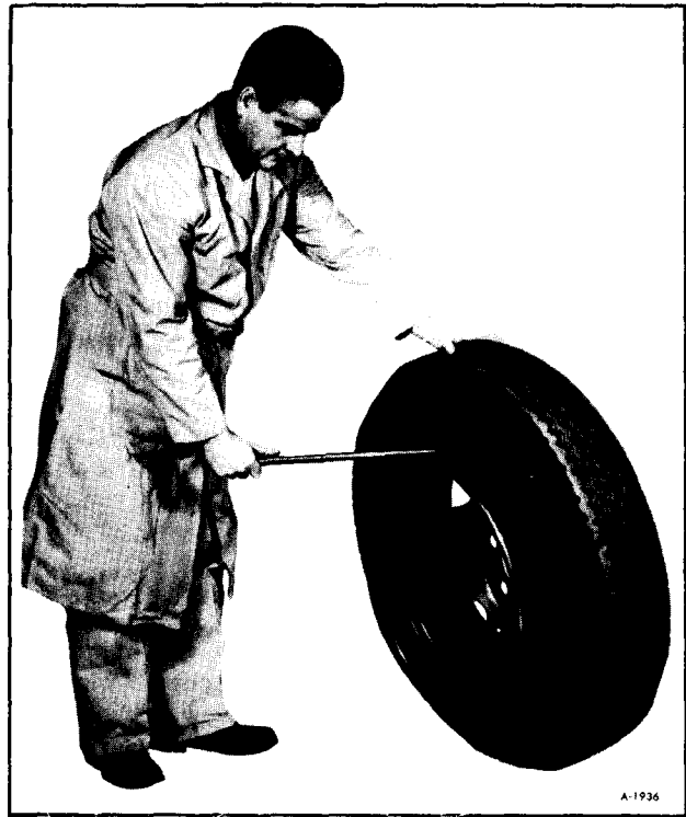
Figure 10—Inserting Tire Iron in Second Bead
