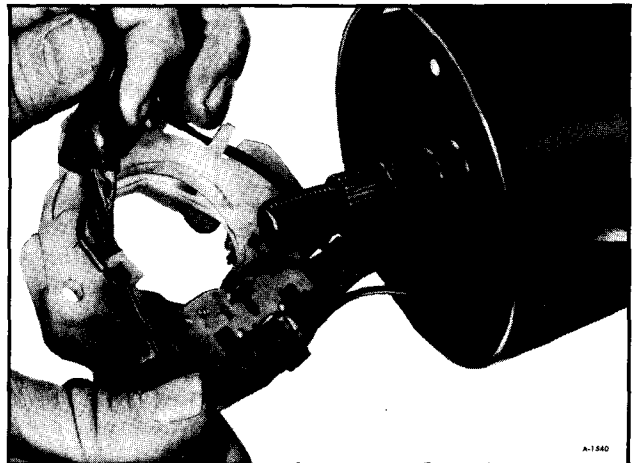
Figure 69—Checking Buzzer Switch Pads
