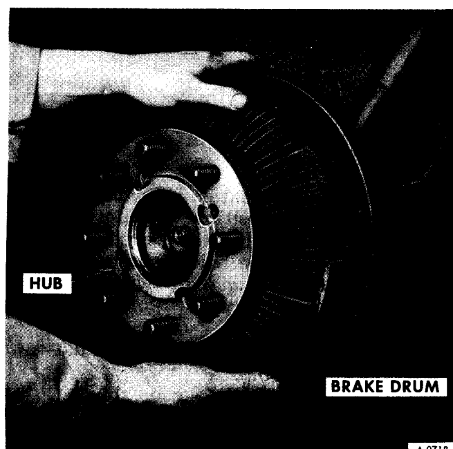
Figure 6—Removing Hub and Drum
