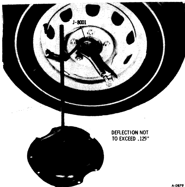
Figure 22—Ball Joint Vertical Check
