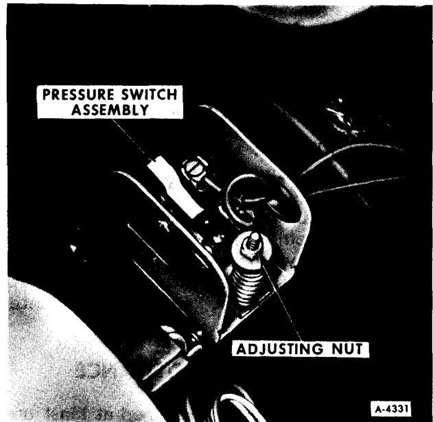
Figure 22—Air Compressor Pressure Switch Adjustment
