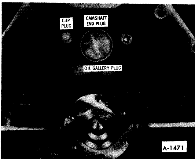
Figure 76—Camshaft and Oil Gallery Plugs
