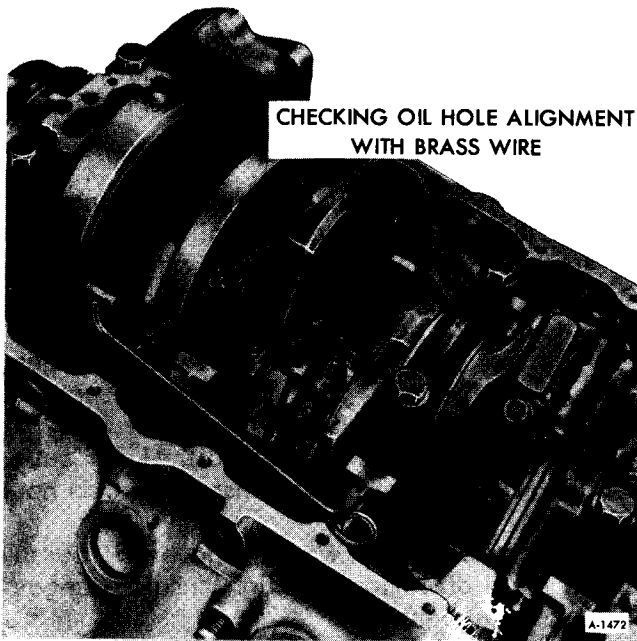
Figure 75—Checking Oil Hole Alignment
