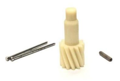
Governor gear repair kit - \$9.99 with free shipping on eBay. Original GM part number 8624939 = K34411A manufactured in USA by Southeast Industries. Includes 2 nails (to pound out old roll pin and install new one – I used a punch instead) and a replacement roll pin. Don't forget to carry a 1/8" diameter drill bit too so that you can drill the hole through this gear for the roll pin installation.
