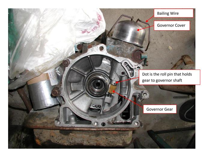
You won't see this view of the inside of the transmission but the photo might help understanding of how things fit together. The bailing wire swivels to the front or rear so that the complete governor assembly from the cover down to the plastic gear can be lifted up and out of the transmission housing.
