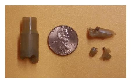
To the left of the penny is the shank of the gear that was still in the governor shaft when we removed the governor assembly from the transmission. To the right are the only pieces of the broken governor gear that I found in the transmission pan after I got home. Perhaps the others were captured in the filter or have not made it to the pan yet.
