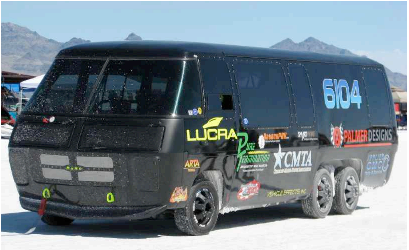
Britt Palmer's modified 1977 GMC Kingsley motorhome powered by a 600 hp Chevy 502 Ram jet fuel injected engine with power transferred through a TH425 transmission. Ran 120.8 mph in 2013 at Bonneville Salt Flats.
