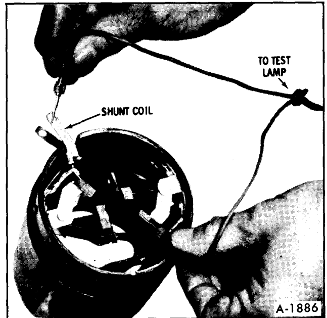
Figure 73—Checking Shunt Field Coil
