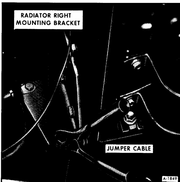
Figure 15—Connecting Jumper Cable to Right Radiator Mounting Bracket
