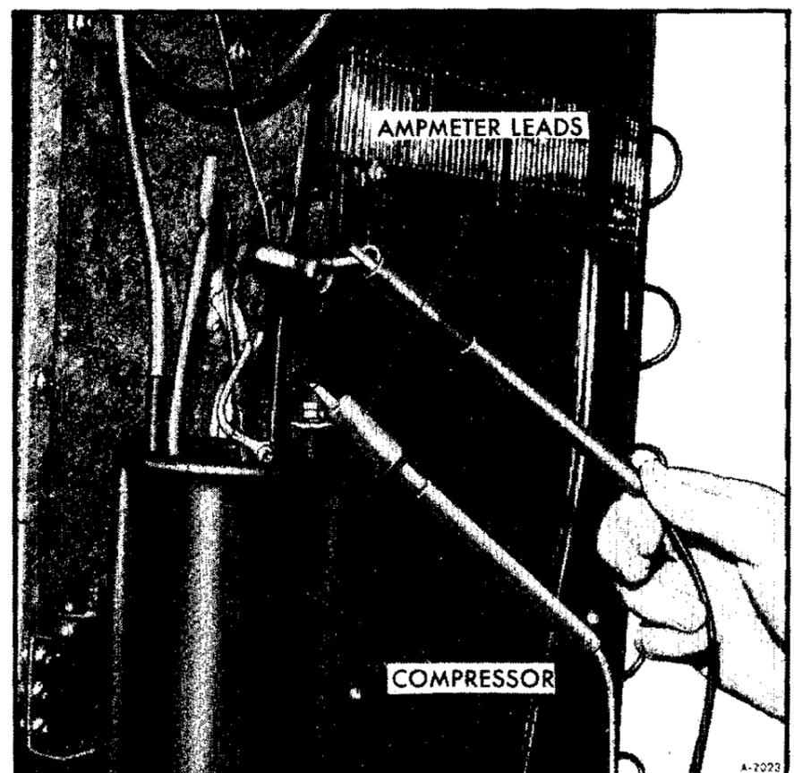
Figure 2—Checking Compressor
