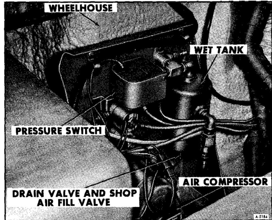
Figure 2—"TWIN BED" Air Suspension Control
