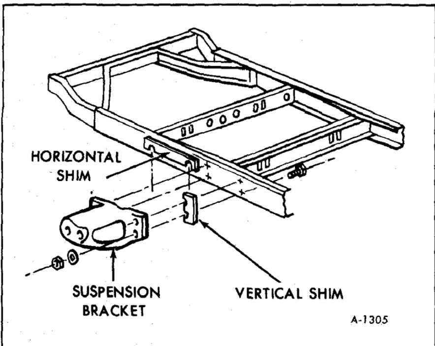
Figure 20—Rear Wheel Shim Location
