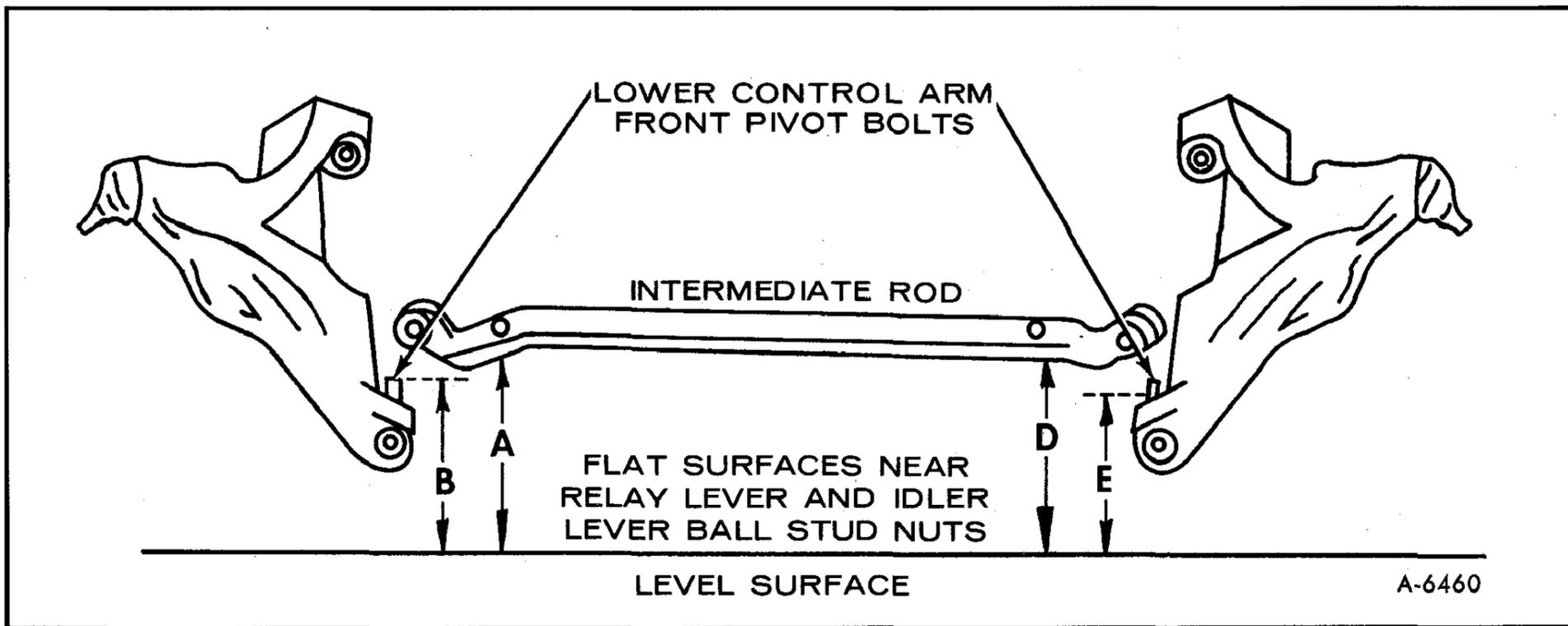
Figure A—Measuring Intermediate Rod Parallelism
