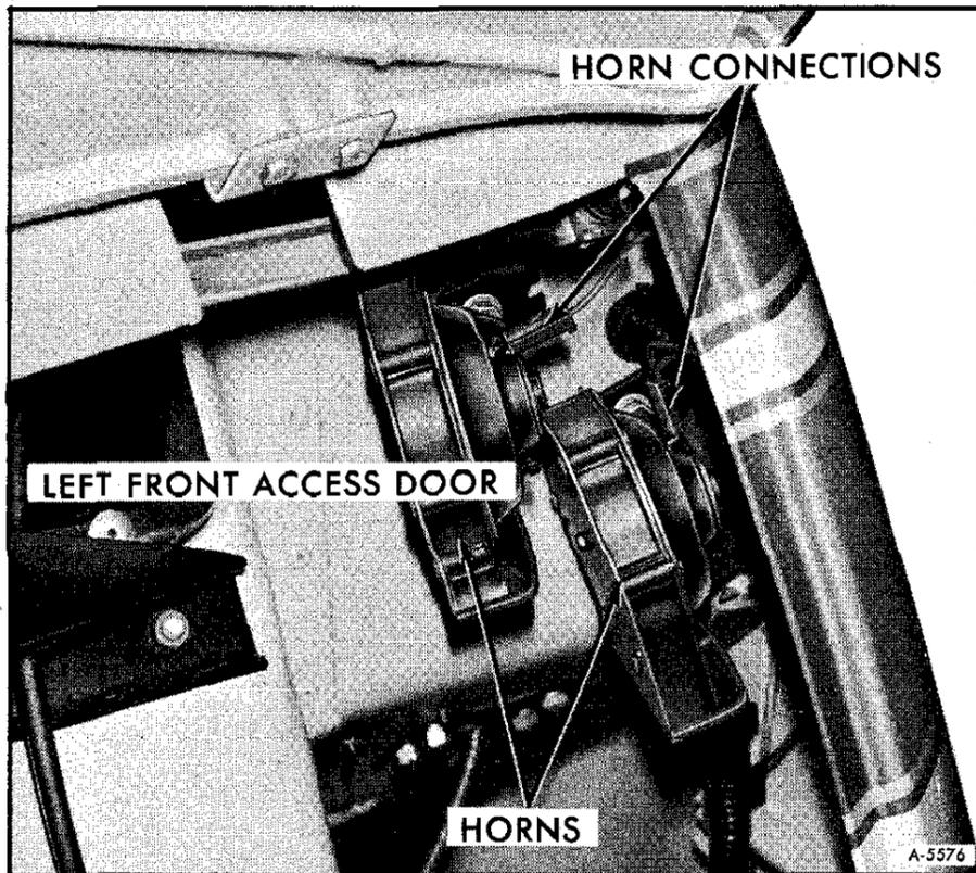
Figure 6—Horn Installation (Typical)
