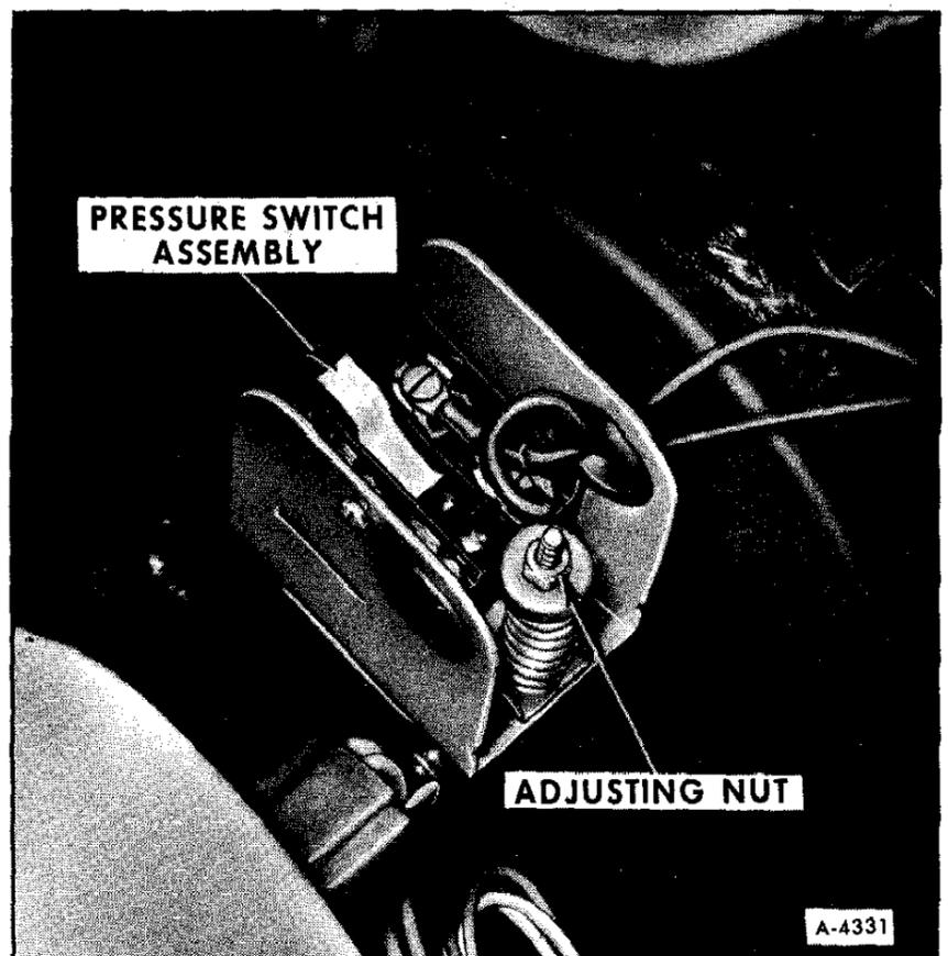
Figure 22—Air Compressor Pressure Switch Adjustment
