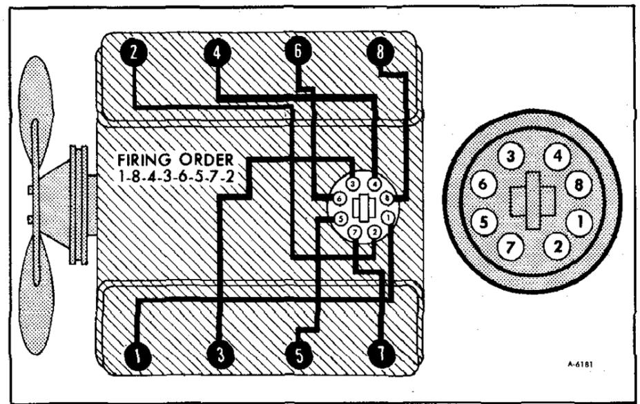
Figure 4A—Secondary Wiring
