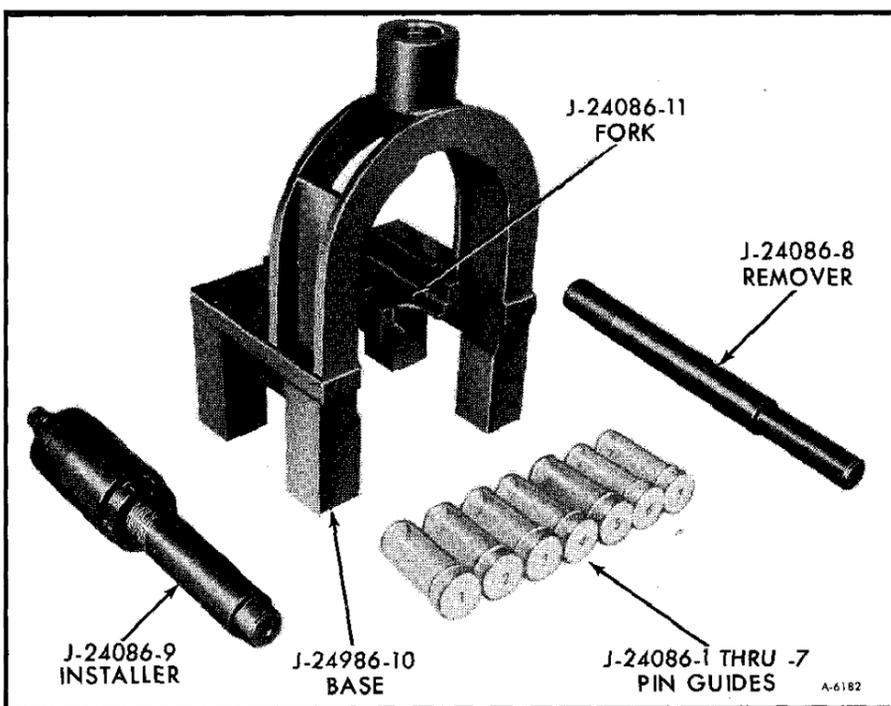
Figure 1—Piston Pin Tool Set J-24086
