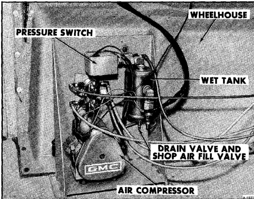
Figure 3—TRANSMODE Air Suspension Control Components,
