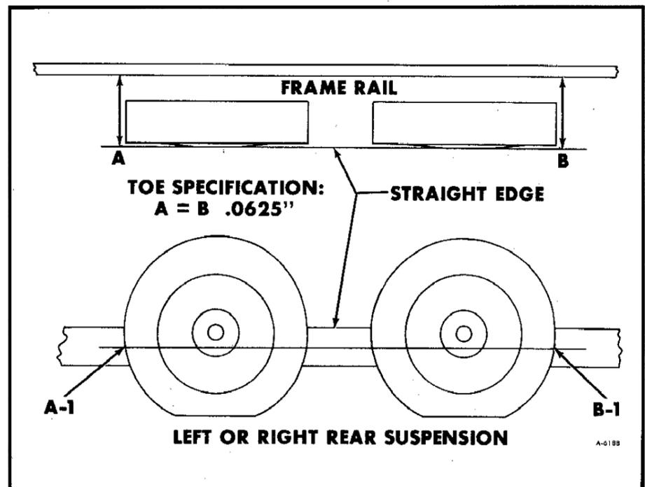
Figure D—Measuring Toe on Rear Suspension
