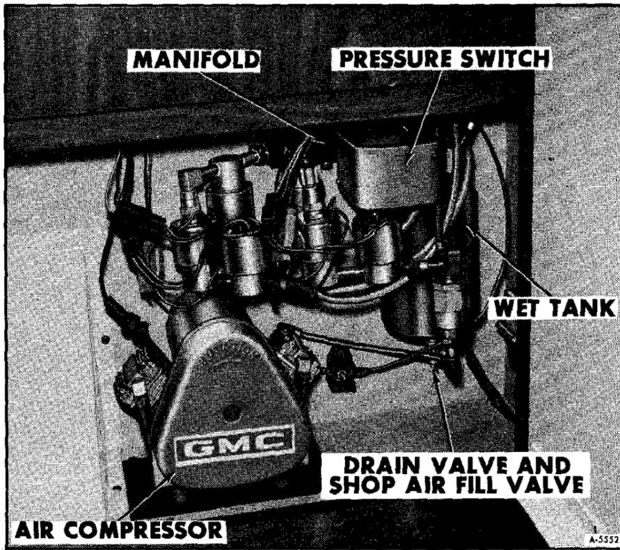
Figure 1—Air Suspension Control Components
