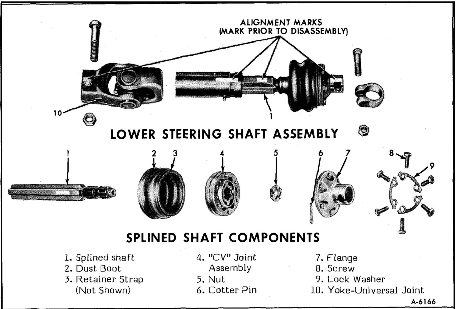
Figure 1—Lower Steering Shaft (Disassembled)
