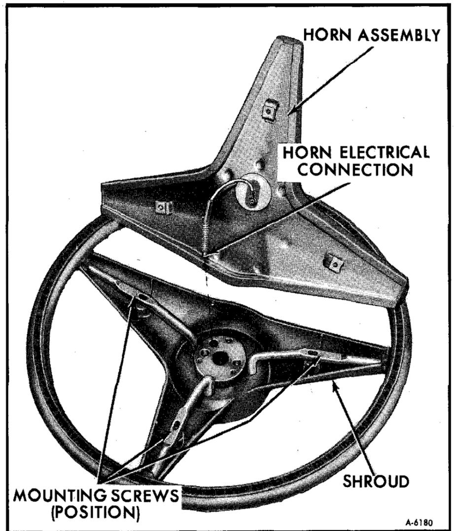
Figure 4—Horn Assembly
