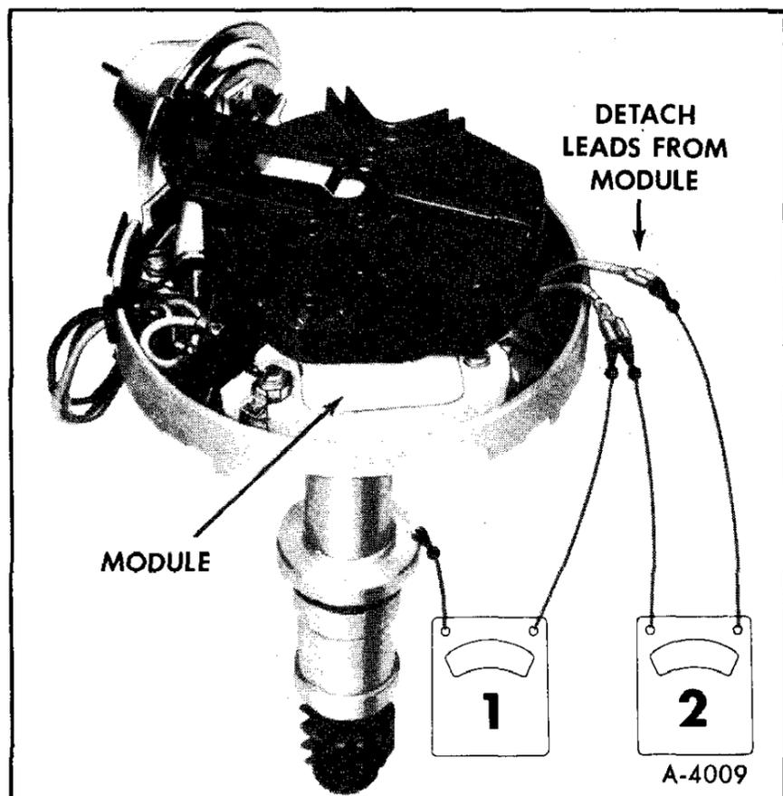
Figure 13—Ohmmeter Check of Pick-Up Coil
