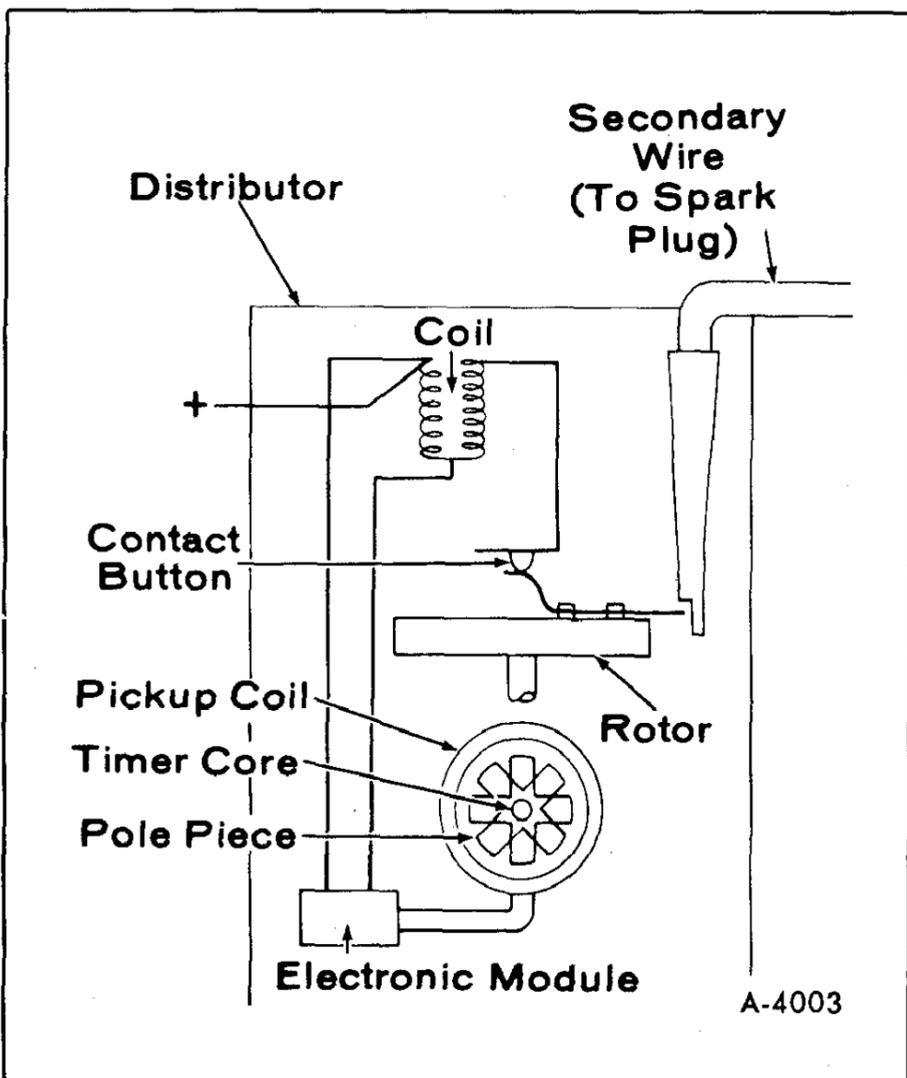
Figure 3—HEI Basic Wiring Diagram
