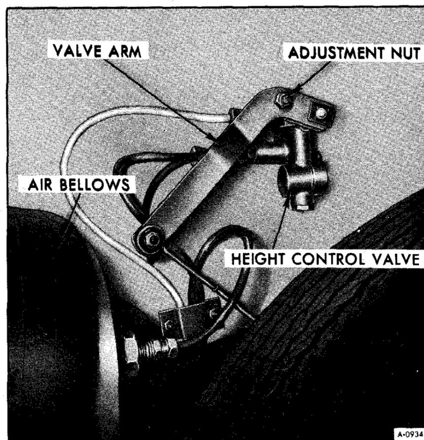
Figure 24—Location for Rear Ride Height Adjustment
