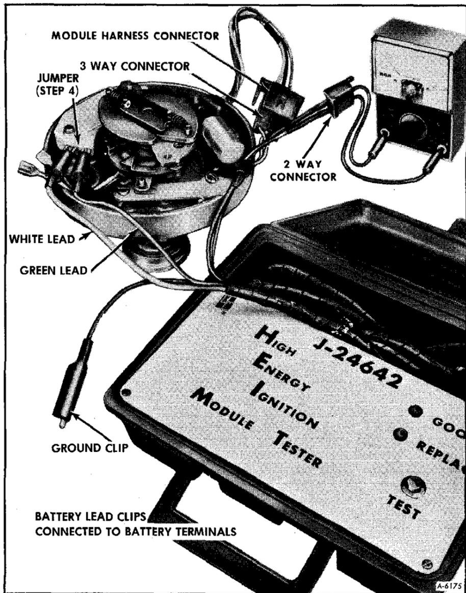
Figure 10—Test No. 2, Using Tool J-24642
