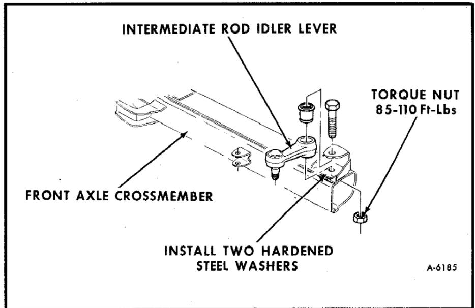
Figure C—Installing Washer Under Idler Pivot
