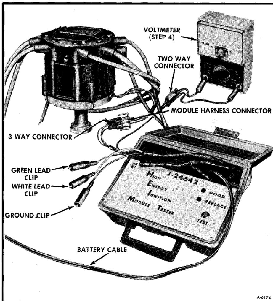
Figure 8—Test No. 1, Using Tool J-24642 (Crank Test)
