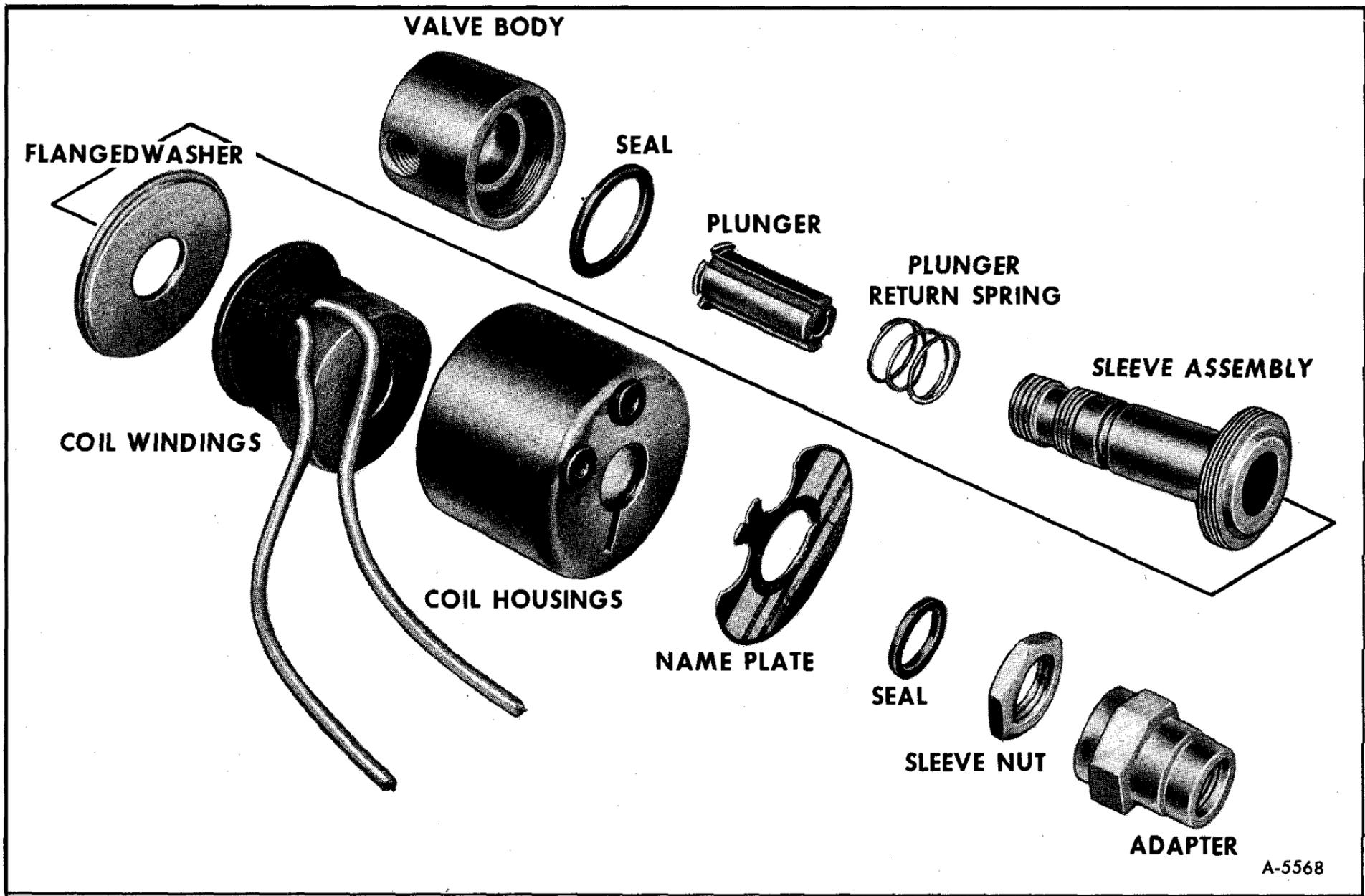
Figure 12—Exploded View of Solenoid Valve
