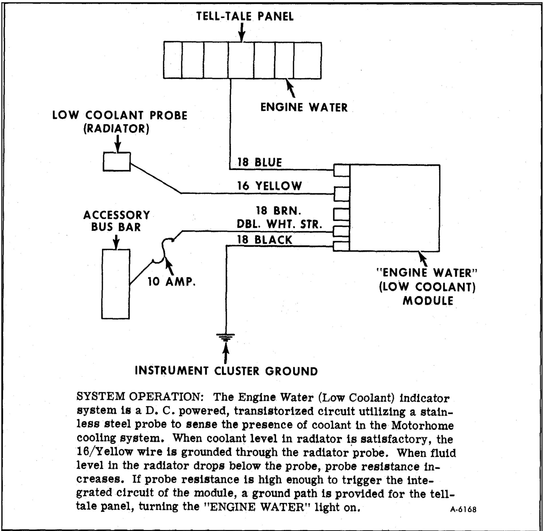
Figure 5—Engine Water (Low Coolant) Schematic
