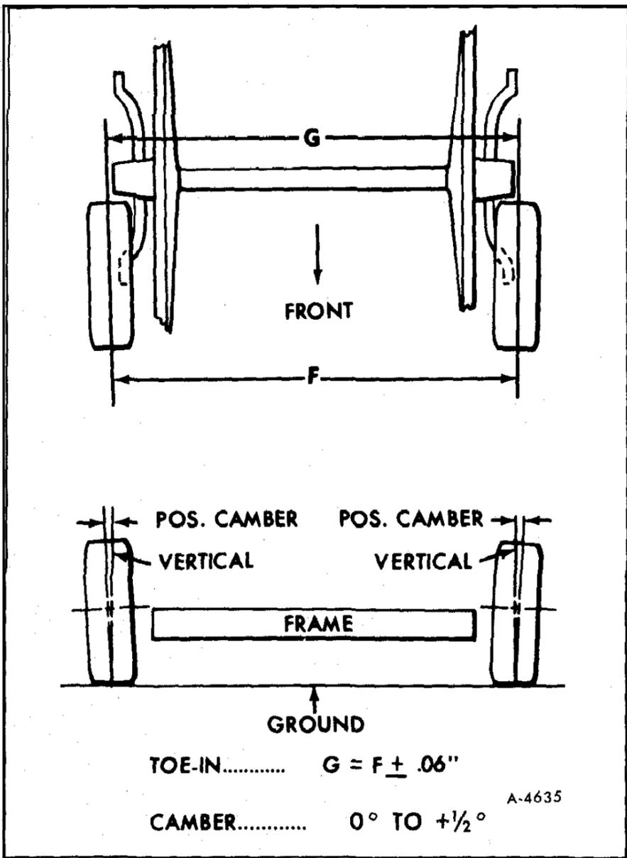
Figure 19—Rear Wheel Alignment Chart
