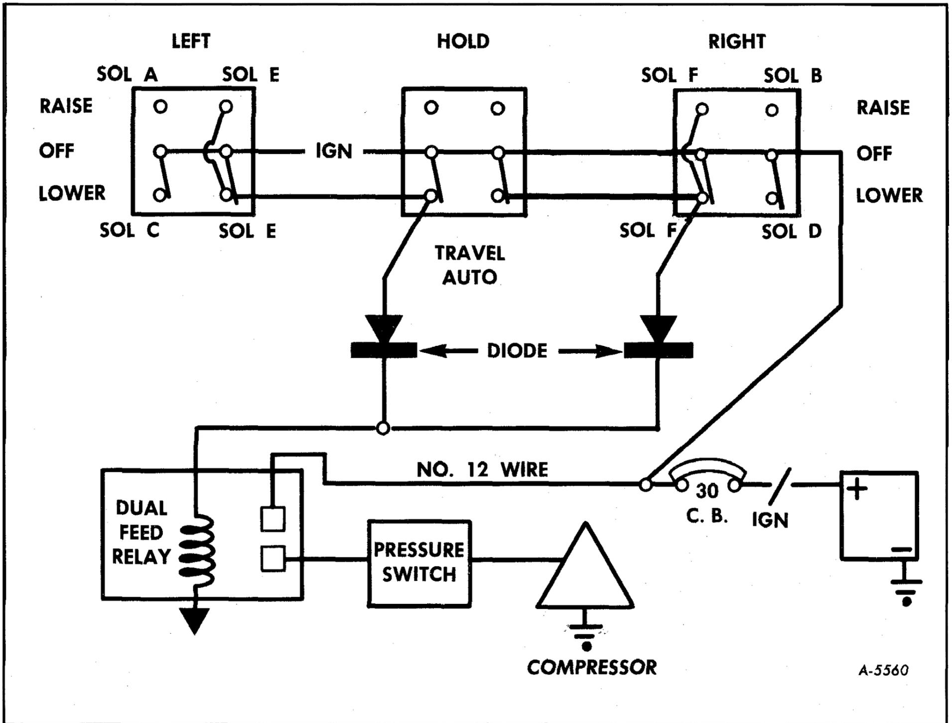
Figure 6—Electro-Level Controls Schematic
