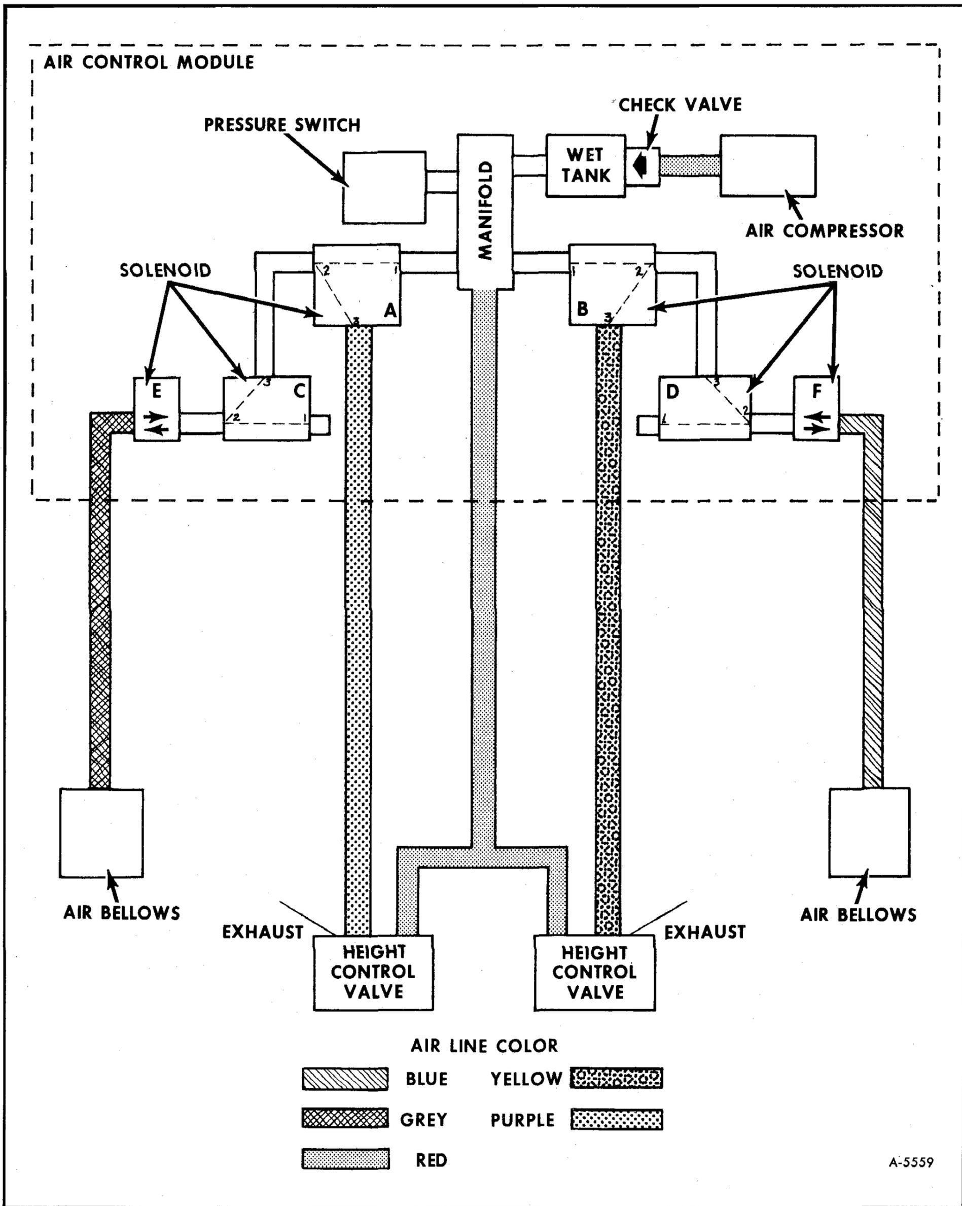
Figure 7—Electro-Level Air Suspension System Schematic
