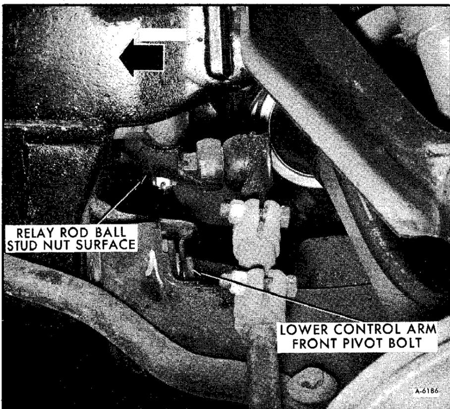
Figure B—Measuring Relay Rod Levelness
