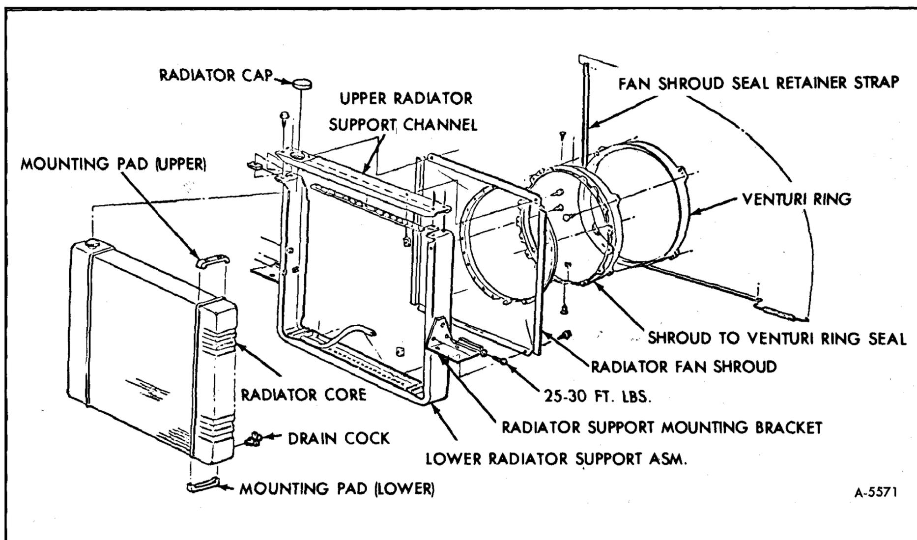
Figure 1—Radiator Assembly (Typical)
