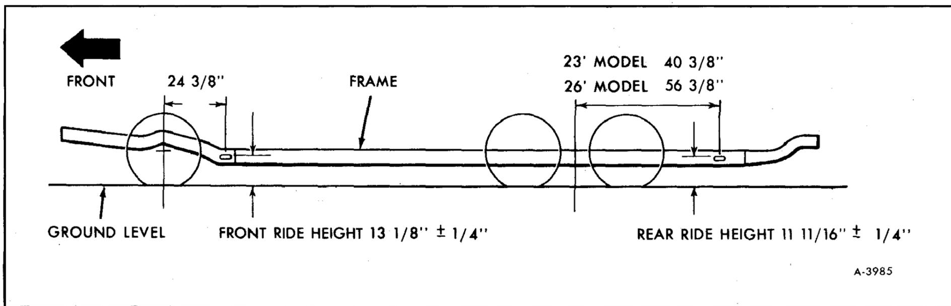
Figure 23—Checking Vehicle Ride Height
