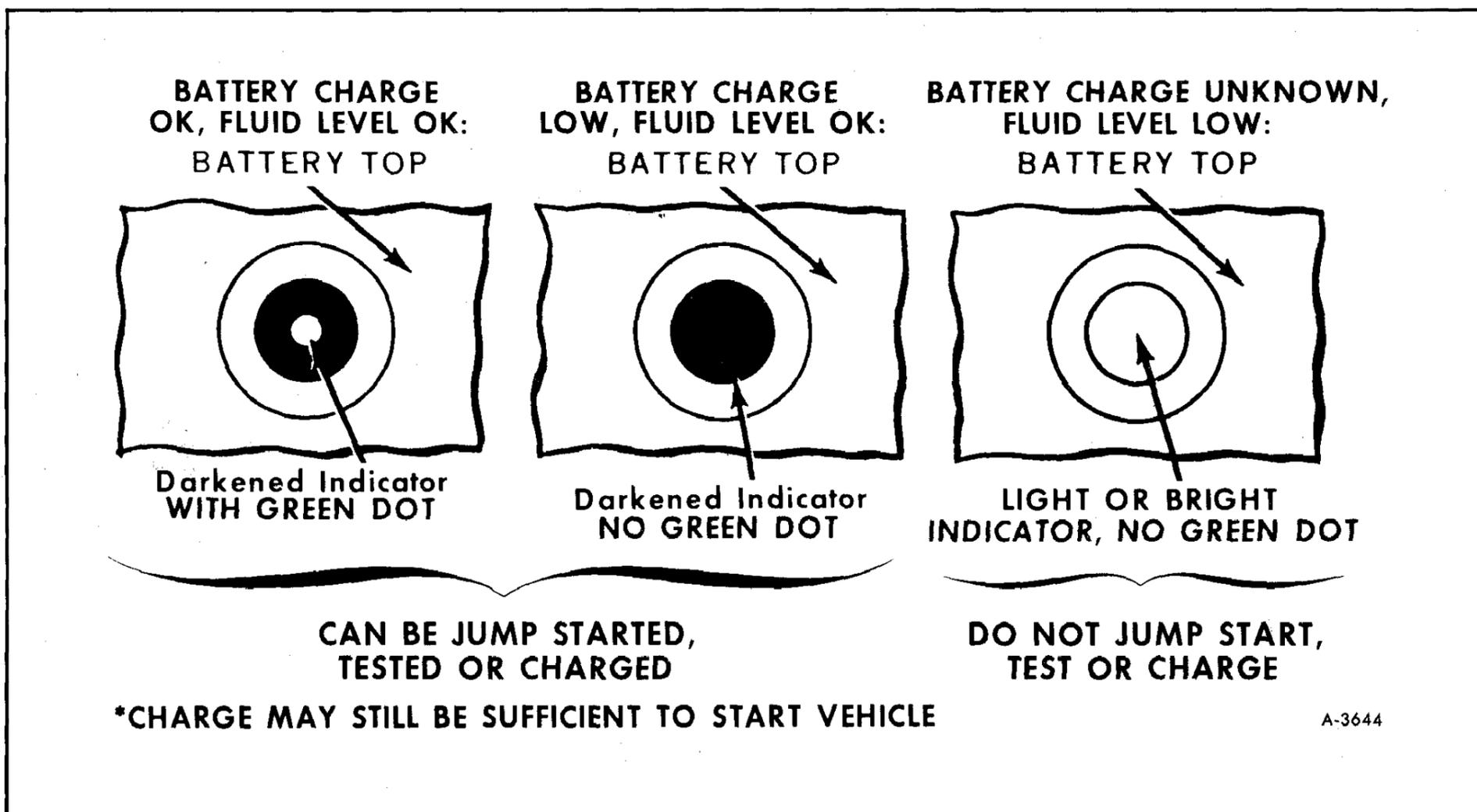
Figure 1—Charge or Test Indicator Conditions (Maintenance-Free Batteries)
