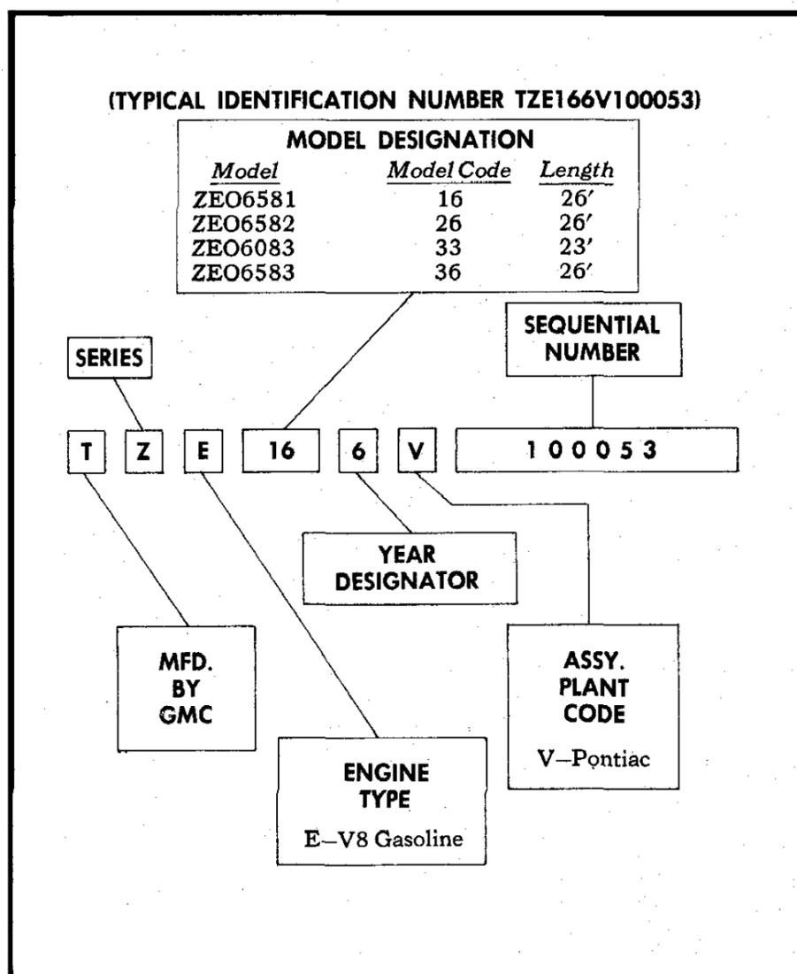
Figure 1—Vehicle Identification Number
