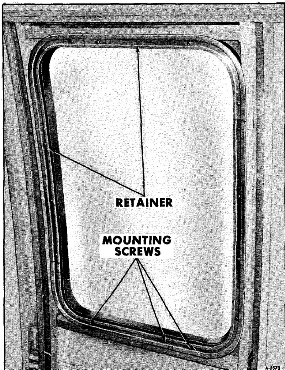
Figure 1—Sash Retainer
