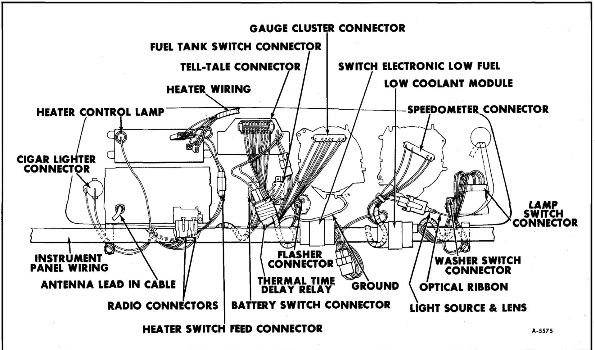
Figure 4—Instrument Panel Wiring (Typical)
