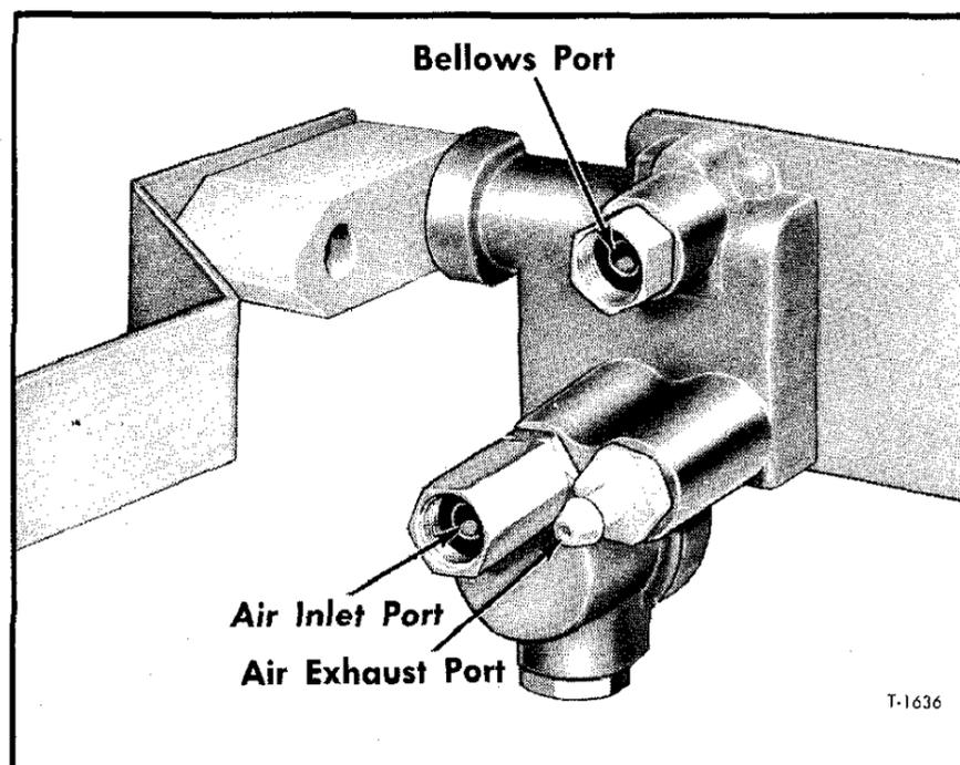
Figure 8—Height Control Valve (Port Identification)
