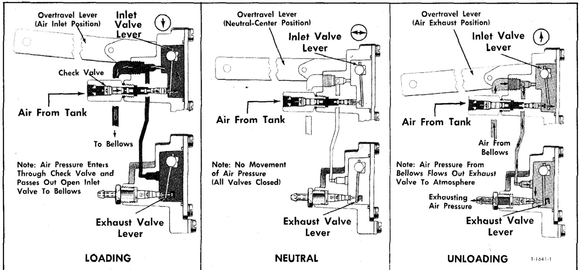
Figure 9—Operation of Height Control Valve
